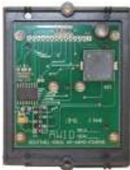
1. KP-6840 keypad assembly, back view, with alignment pins.
