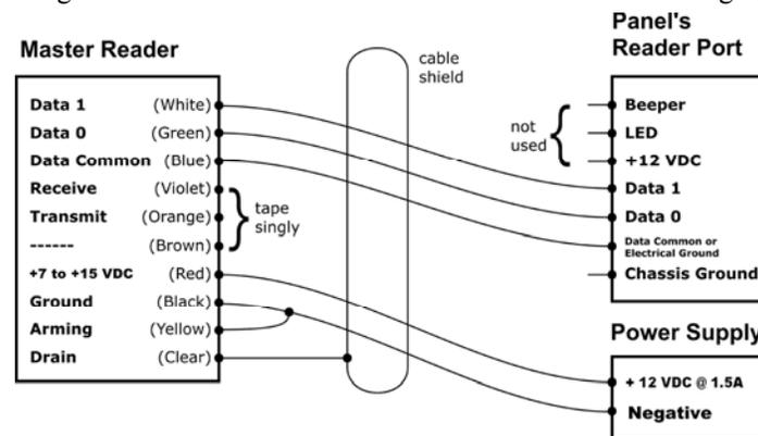
Figure 3. Wiring the Complete System for Wiegand Interface
