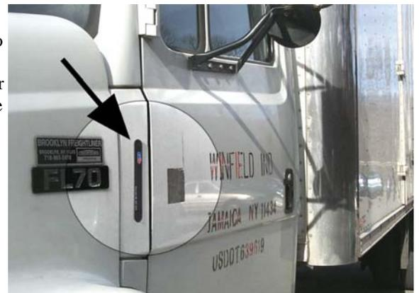
**Figure 2. MT-1014 tag on side of truck cab.**
